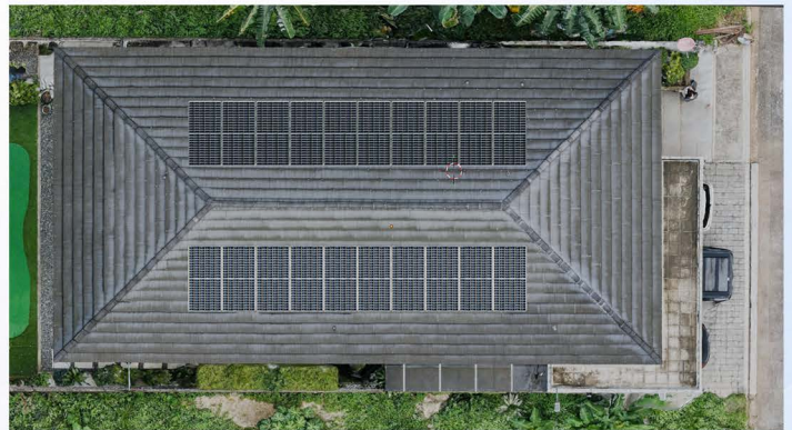
ROOF-MOUNTED SOLAR ARRAY LAYOUT
